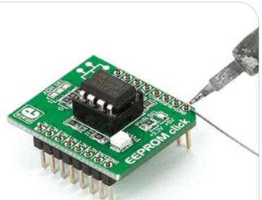
Turn the board upside down so that bottom side is facing you upwards. Place shorter parts of the header pins in both soldering pad locations.
