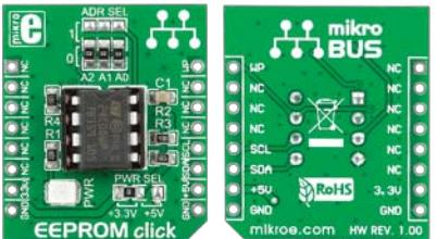
EEPROM Click™ is an accessory board in **mikroBUS™** form factor. It's a compact and easy solution for adding more EEPROM memory to your device. It features DIP 8 **24C08** 8kbit serial EEPROM module in DIP 8 socket. EEPROM Click™ communicates with target board via I<sup>2</sup>C interface. The board is designed to use 3.3V and 5V power supply. It has a LED diode (GREEN) that indicates the presence of power supply.
